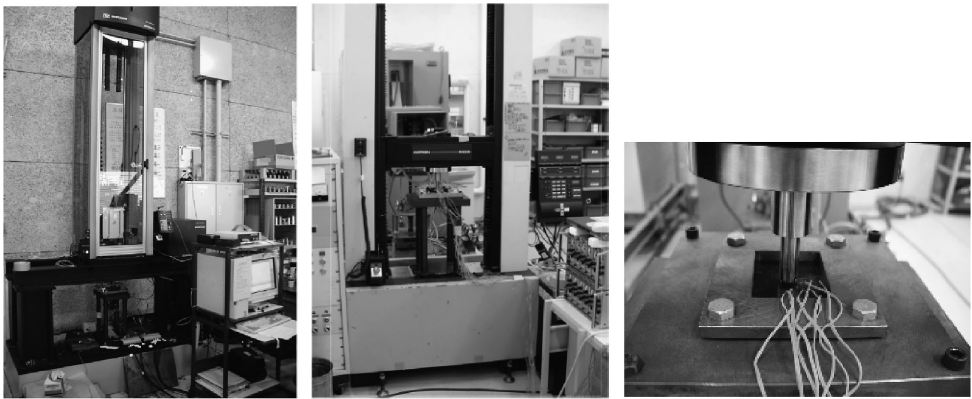
(a) Impact test machine (b) Static indentation test machine (c) Support fixture
